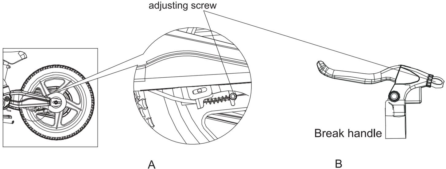
If the braking distance increases or the braking force decreases. Please check immediately, and use a wrench to unscrew the adjusting screw to increase the pre-tightening force of the brake cable, as shown in Figure A; or fine-tune with the adjusting screw shown in Figure B
