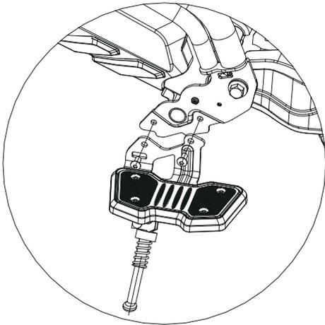
Use M4 hexagon socket wrench to install the pedal
