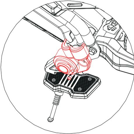
Install the outside plastic cover using an M3 inner hexagon wrench
